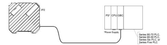
Figure 3 - 3. PLC/Panel Connection
